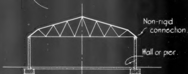
FIGURE 6: TRUSS RESTING ON TWO SUPPORTS.
