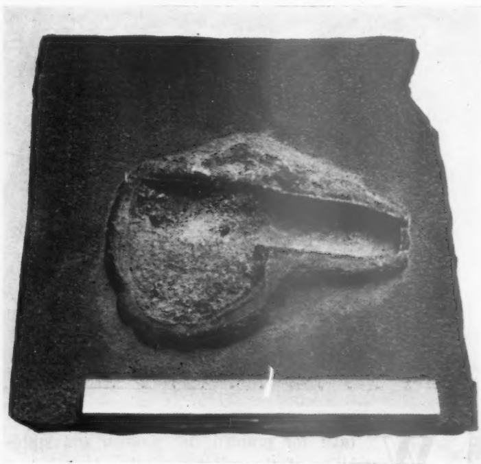
"An area of asphalte cut out from a roof showing the imprint made by a kilo incendiary bomb. The asphalte was not penetrated either by heat or impact."
