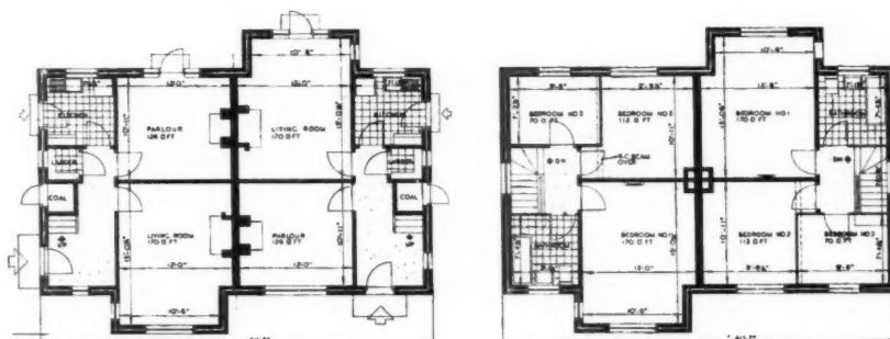
Main elevation and ground and first floor plans of B 3a type house.
