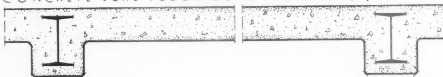
HOLLOW BLOCK FLOOR CONSTRUCTION (reinforcement not shown)
