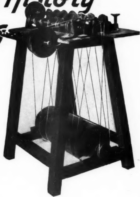
This machine made and used by W. T. Henley over a hundred years ago will still cover fine wires with silk and cotton with unimpaired efficiency.
