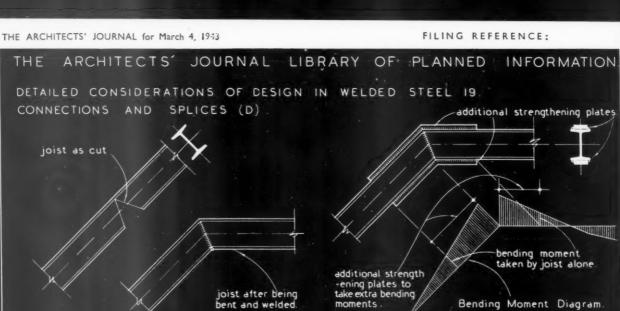
FIGURE 1: WELDED CORNER OF ARCHED FRAME OF R.S. J. SECTION
