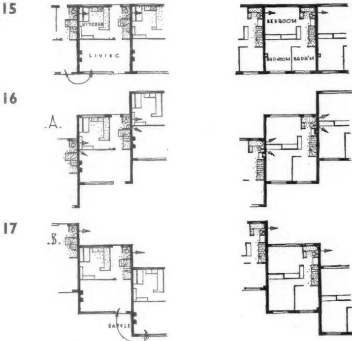
15, 16 and 17 show the advantages gained by suitably staggering a terrace type plan which would have objectionable features in terrace form. A in 16 gives no advantage. B in 17 indicates the best method.
