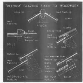
"REFORM" Roof Glazing has been consistently improved over a period of some sixty years during which time it has found increasing favour on account of its scientific efficiency, economy and durability. It may be applied to new or existing roofs of any type. Particulars on request.
