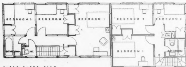
Above, the job nears completion. Note the brickwork on the garden elevation. Brick is a possible cladding material as well as local stone. Below, ground and first floor plans of the houses at Hendon designed by F. R. S. Yorke. The grid dimension used throughout is 3 ft. 2 in.
