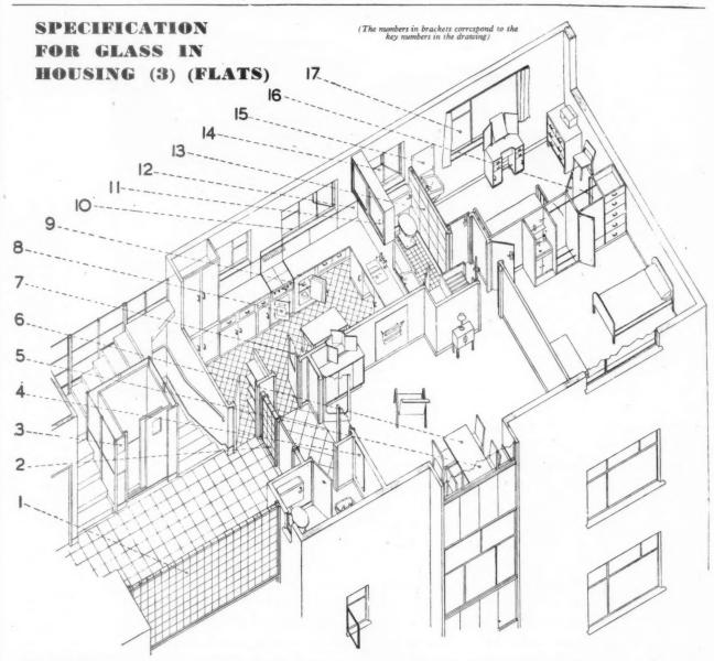
**STAIRCASE PANELS**: (I) Insulight hollow glass bricks: fire-resisting glazing with thermal and sound insulation.
