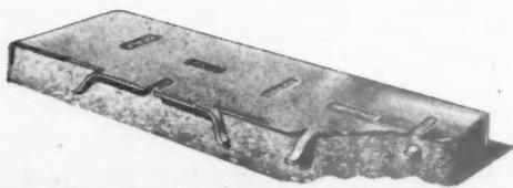
Section of a Stelcon Anchor Steel Plate showing how firmly every 3 square inches are anchored to the concrete sub-floor.
