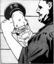
7" Heavy Duty Sander removing shuttering marks from poured concrete.
