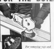
For removing rust and scale use B & D Sander with cup wire brush.
