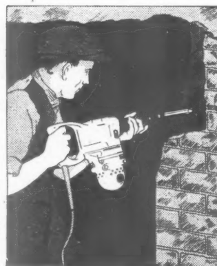
Breaking through brickwall with No. 36 Hammer and bull point.
