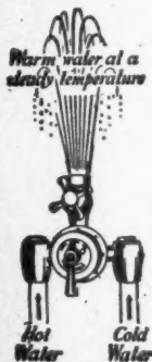
Leonard-Thermostatic hot and cold Water Mixing Valve serving wash-basins.
