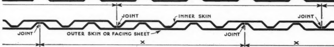
SECTIONAL PLAN SHOWING POSITION OF JOINTS
