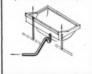
MAINS SUPPLY, HOT BRANCH AND WASTE TO SINK (E.M. ITEM 8 & NOTE 'b')
