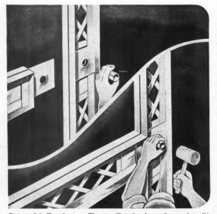
Diagram of the Trusteel system. The upper illustration shows a beam ready to slide into place in the stanchion on the mortice and tenon principle. The lower illustration shows the beam in position with the tubular steel pin being inserted. See No. 2644.
