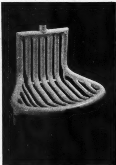
The Rad-Vec grate, a variation of the common back boiler taking the form of a small water tube unit of welded pipe, will feed radiators at the same level or on upper floors to provide back ground heating.
