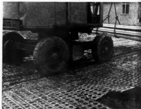
Three photographs exemplifying some of the work of the Building Research Station. Top, apparatus designed for studies of rain on roofs; the slope of the roof can be altered and the rain can also be driven by a wind. Centre, measurements being made of the deflection under vertical load, of a steel frame for an alternative form of house construction. Bottom, study being made of temporary air-stripping for housing sites to keep them reasonably clean during construction.
