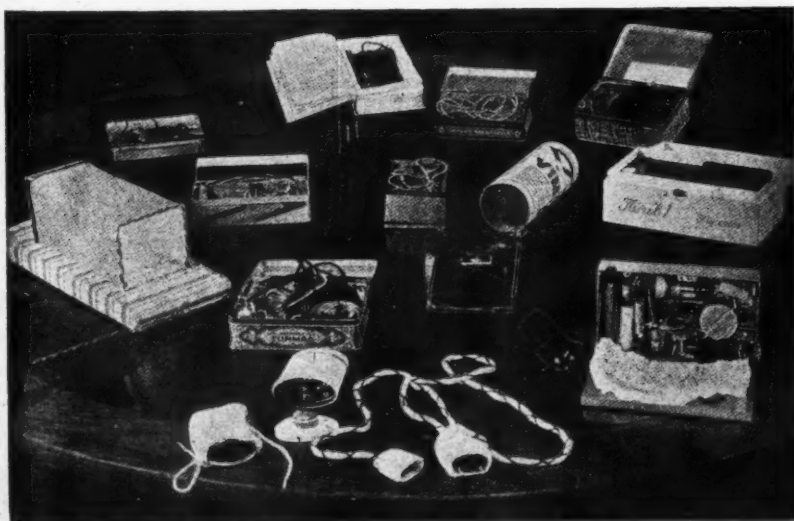
Disguised radio receiving sets made secretly in occupied Holland. See Astragal.
