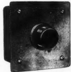
A single service Group Lamp Unit, flush fixing, with projecting cylindrical lamp giving maximum visibility. Dimensions: Front-plate, 4" x 4"; Box, 3 1/4" x 3 1/4" x 1 3/8".
