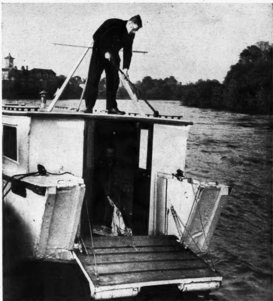
Right: the floating home is boarded by a hinged ramp leading through French doors to the two-berth fore cabin illustrated on the following page. Bottom, a general view showing the ramp in a lowered position.
