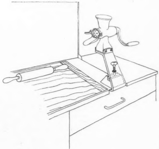
Fig. 4. Top of a kitchen cupboard unit by Weldall & Assembly, Ltd. The bracket for the mincer is quickly detachable. (Stand N 247.)
