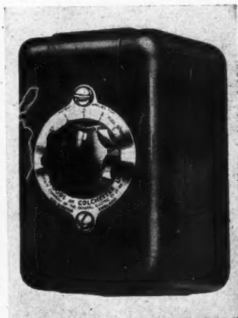
GEC speed regulator for propeller fans giving a downward speed regulation of 30 or 40 per cent. with either 4 or 5 running speeds, and "off" controlled by means of a snap action switch.
