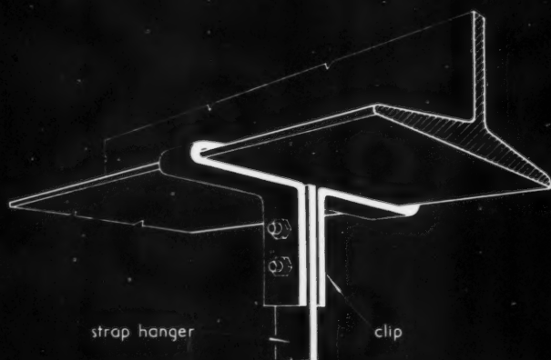
SUSPENSION FROM BOTTOM FLANGE OF R.S.J.
