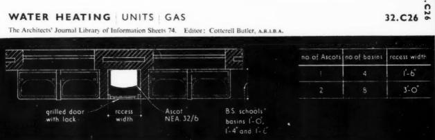
H.W. SUPPLY TO BASINS BY ASCOT NEA. 32/6 MULTI-POINT HEATER IN RECESS WITH PROTECTIVE GRILLE.
