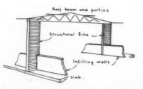
The diagram illustrates the principle of framed construction with panel walls referred to in the article.
