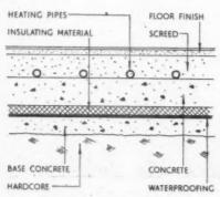
Construction for floor heating.
