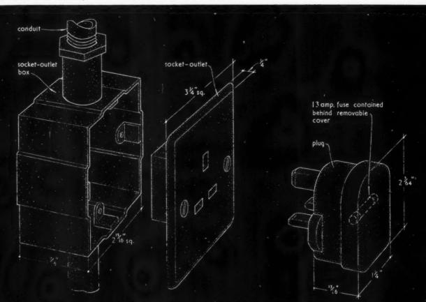
13 AMP. FUSED-PLUG AND SOCKET OUTLET SUITABLE FOR RING MAIN CIRCUITS (TO B.S. 1363).
