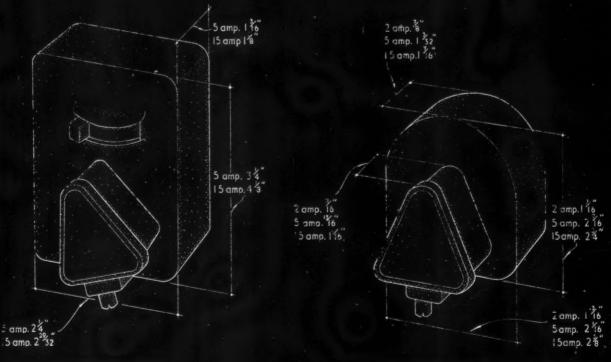
5 AND 15 AMP. SHUTTERLOCKED SAFETY SWITCH SOCKETS. 2,5 AND 15 AMP. SAFETY SOCKETS. (TO B.S.546).
