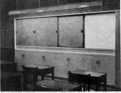
An example of how brightness concentration, of the kind referred to in the article, can focus attention on important points in the room. Here, fluorescent lighting over the blackboard gives a comparatively great light intensity in comparison with the rest of the room. The classroom is one in a school at Ruislip by Howard Lobb.
