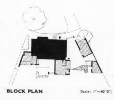
The part of the house at present under construction is drawn in black; proposed additions at a later date are hatched.
