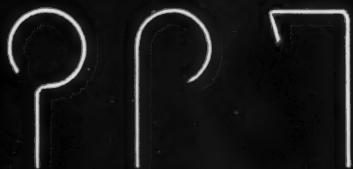
ALTERNATIVE ROLLS FOR EDGES OF GUTTERS.
