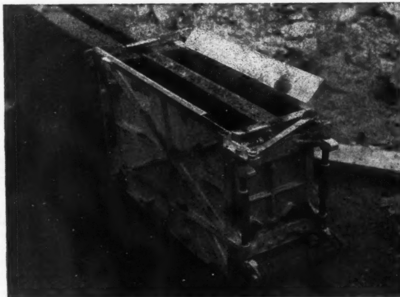
Hyspecon walling machine, a temporary formwork unit for the production of 9 in. walls with a 2 in. cavity in sections 2 ft. 6 in. long by 1 ft. 3 in. high. The equipment consists of three forms: the one illustrated here, a corner unit with a continuous cavity, and a further unit for producing 4 in. solid walls.
