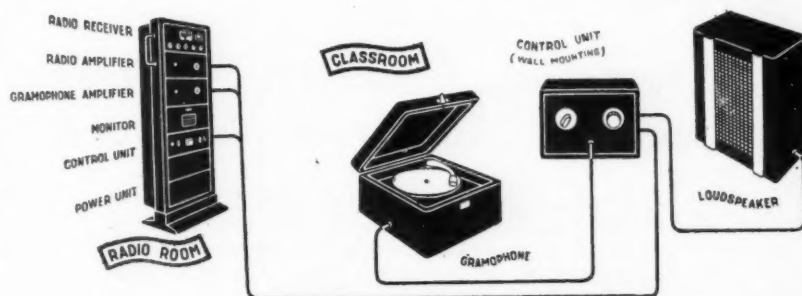
Above, a radio installation in which both the receiver and amplifiers are housed in a room separate from the classroom. Right, gramophone reproduction in the classroom.
