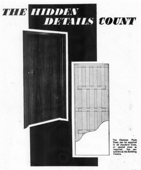
On the surface there is little to distinguish the Chelmer semi-solid fiush door from the standard hollow-core type. It is the hidden details of design and construction which account for its superiority the laminated frame, the additional vertical members tenoned and glued into the rails, the precision of
