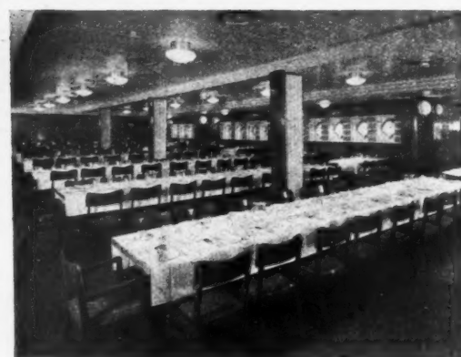
Above, the first class café. The screens are of bamboo. Other woodwork is of zebrawood. The chairs are of bleached ash, with plastic tops to the tables. Below, a detail of the first class dining saloon. The floor is cork linoleum. Woodwork is in bleached mahogany and ash. Furniture is of beechwood, and is upholstered in plum-coloured hide.
