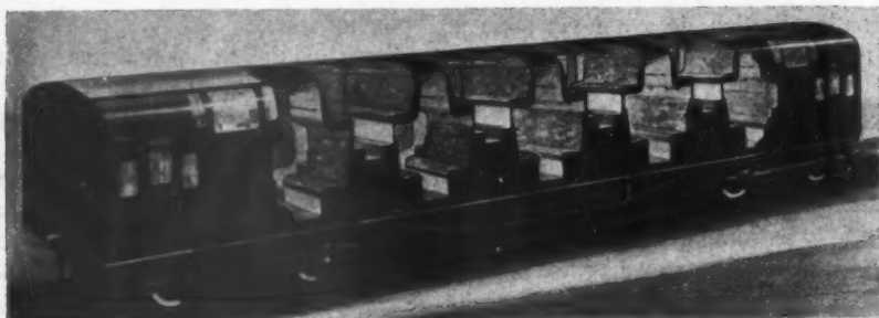
A cutaway section of the proposed double-decker coach, for suburban lines of the British Railways. See Astragal's comment below.
