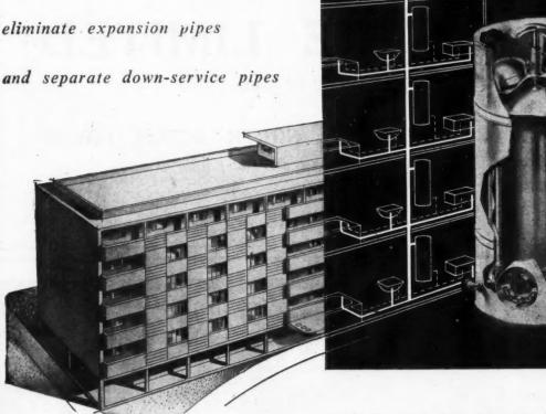
O SIMPLIFY building plans and save material, Sadia engineers have designed two new water heaters especially for use in blocks of flats. One is all-electric, the other is coal-electric. In each type, the cold water is supplied to the storage heater from a self-contained ball-valve tank which is built into the unit itself.
