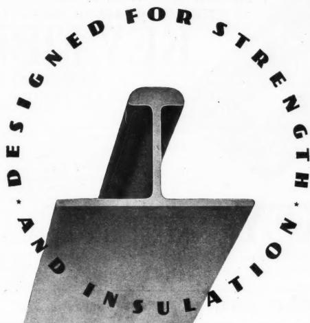
This new Sundeala Aluminium Alloy Tee Bar uses the well-known 'V' clip method of Board-retention. The unslotted, flanged-head Tee Bar lends itself admirably to the extrusion process of manufacture and the flanged head has been developed to give maximum strength. The seamless base (only .05" thick) provides an improved and unobstrusive panel border. Trimming members (Tee noggings, Channels, Angles, etc.) are also available in alloy.
