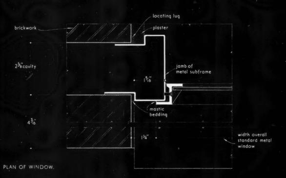
STANDARD METAL WINDOWS WITH STEEL SUBFRAMES: FIXING TO II" CAVITY BRICKWORK, (scole 2 full size) Compiled from information supplied by The British Metal Window Manufacturers' Association Limited.
