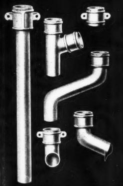
'Birmid' R.W.G. are light but very strong with the result that breakages in transit and on site are almost unknown. The rainwater pipes are made of extruded and drawn material, although under one eighth of an inch in wall thickness they are stronger than any other material used for this purpose. These pipes can be had in all lengths up to 18 feet. Further particulars are given in the new price list which is now available. If you have any doubt or reservation
