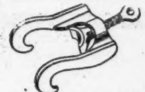
BRACKET WALL FORM CLAMP. For fixing Scaffold Brackets, Eaves, Brackets and Tube Runners to Wall Forms. One screw fixing. Sheradised throughout.
