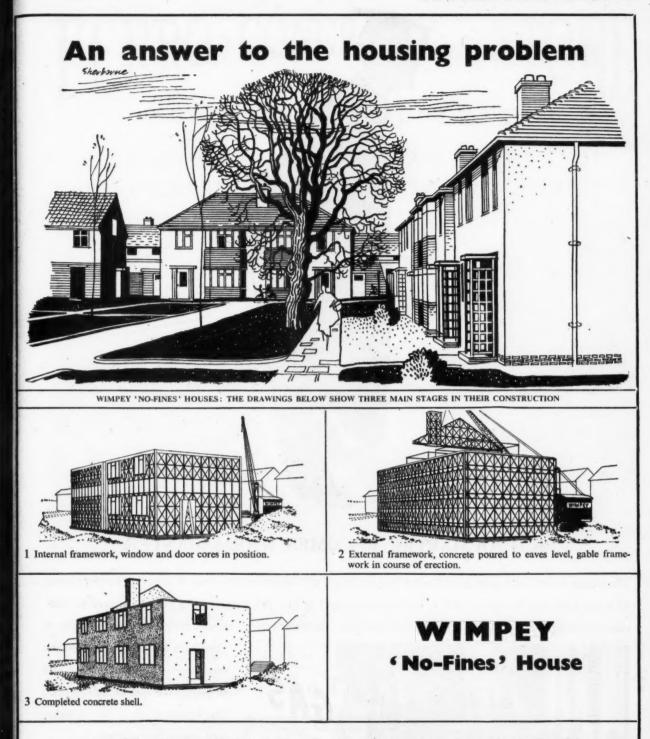
BY APPLYING civil engineering methods to the housing problem Wimpey's have evolved the *No-Fines* house —warm, solid, permanent, quickly and economically built.
