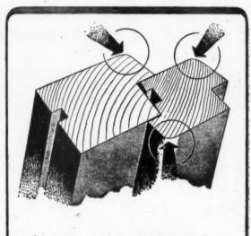
The rounded arrises illustrate a characteristic Ripper refinement of finish.
