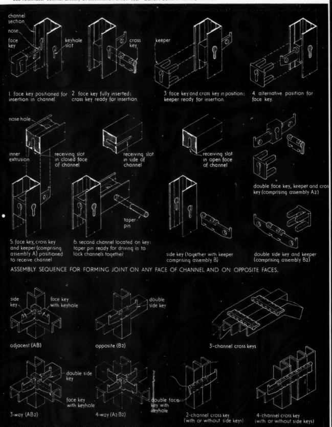
TYPICAL JOINTS TO ACCOMMODATE TWO OR MORE CHANNEL SECTIONS.
