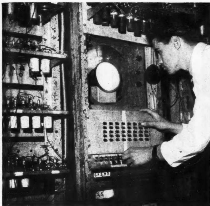
Part of the mechanical brain at Manchester University, designed by Professor F. C. Williams and Dr. Thomas Kilburn. See Astragal's comment below.
