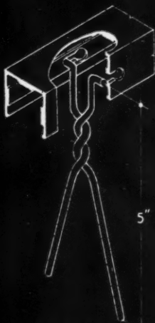
LOCATION OF TIE IN CHANNEL PERFORATION.
