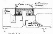
SECTION [Scale:  $\frac{1}{2}{}'' = 1'0'$ ] DETAILS OF FLOOR EXPANSION JOINTS
