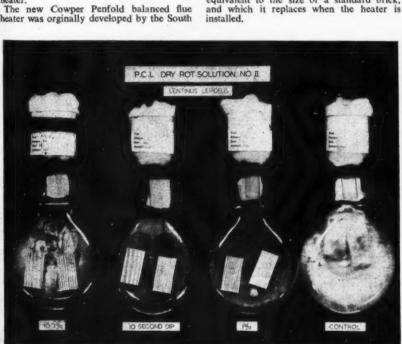
Tests carried out at Princes Risborough on P.C.L. No. 2 dry rot preservative. The flask on the right holds the untreated specimens. The fungus used for the test is more resistant than merulius lacrymans. All the flasks have been in an incubator for three months.
