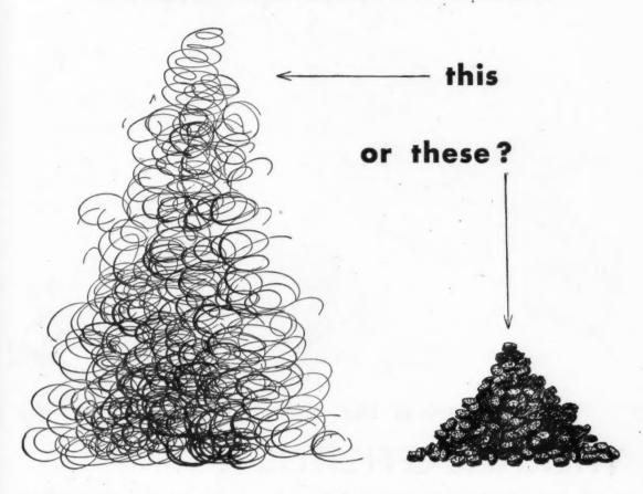
The briquetting of iron, steel, brass, copper and aluminium borings and turnings transforms loose and bulky material into dense blocks equal to lump metal. Handling is facilitated, storage is brought down to a minimum and remelting losses are reduced to that of virgin metal. The 'Emperor' Press, illustrated below, is equally efficient in briquetting coal dust and other fine pulverent materials. Full details of the 'Emperor' Press and other
