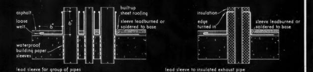
LEAD FLASHINGS TO ASPHALT AND BUILT-UP BITUMINOUS SHEET ROOF COVERINGS.
