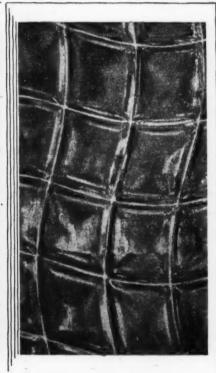
**ARGENT** Average diffuse light transmission is 75%. Power of diffusion and obscuration is very high. This pattern has a bright scintillating appearance.
