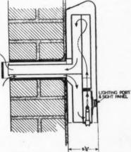
The Cowper Penfold balanced flue heater, top, and bottom, a section of the heater showing the external air duct.
