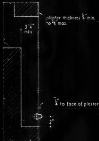
SECTION THRO' FIRE SHOWING SPECIAL FLUE NOZZLE FOR USE WITH NAUTILUS FLUE (MODEL 7505 ONLY).
