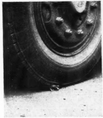
A Sanders unbreakable plug showing distortion produced by the weight of a 7½ ton bus.
