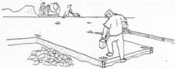
1. Site slab is poured with deepened slab at edges and reinforced to form an edge beam. Forms are left in at stanchion position and later removed to form mortices for the holding down bolts.
