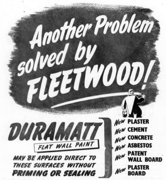
**DURAMATT** is unaffected by the chemical action in any of these materials and allows contained moisture in the walls to come through without risk of saponification or flaking. Efflorescent salts can be washed off without damaging the paint film.
