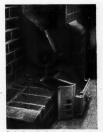
Sectional model of one of the new fuelsaving grates on the stand of the Coal. Utilization Joint Council.
