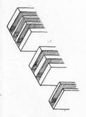
Isometric sketches of Pilkington's Insulight glazing units. The double-glazing unit was described last week; the treble and quadruplicate units are used where a specially high degree of insulation is required as in refrigerator show cases or thermally controlled laboratories.
