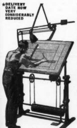
The MAVITTA Drafting Machine stamps your drawoffice as EFFICIENT. Made of steel tube with adjustable ballbearings. The main angles are located automatically, intermediate angles by lock. Scales have inlaid celluloid edges and are divided to order on two edges.
