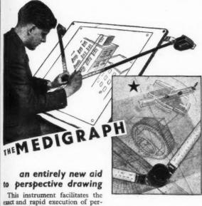
spective drawings. It provides positive location of vanishing points outside the drawing board, and car-ries a series of scales with which foreshortened dimensions can be instantly plotted. These features diminate the involved projections necessary when ordinary orthographic instruments are used-
