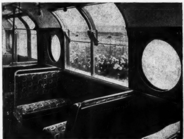
This tube car, which has been put into operation on the Bakerloo line in London, is a converted car of the present standard pattern. A high window line has been provided to give more light for passengers.
