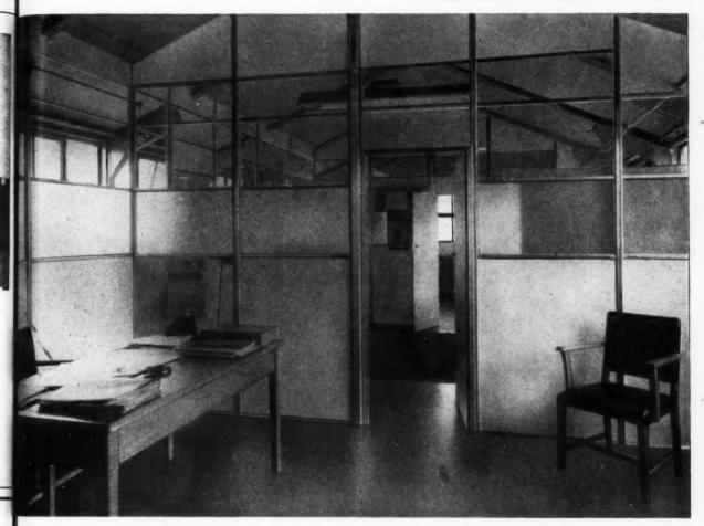
meal view of offices of K. L. M. Royal Dutch Airlines, at London Airport, designed by J. Stroud Foster, A.R.I.B.A. Conversion of concrete hut executed by Compactom Ltd., with partitioning of "PLIMBERITE" and glazing in aluminium framing.
