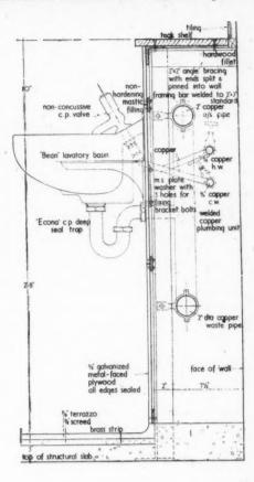
Above, typical detail of men's lavatories showing large duct to accommodate pipework; trough type water waste preventors are also used and are placed in the duct. [Scale:\frac{1}{2}''=1'0'']. Right, detail showing "Bean" lavatory basin with "Econa" c.p. deep seal trap. The basins are fixed direct to metal faced ply covering and a preformed welded copper plumbing unit. The two drawings have been made from working drawings kindly lent by the Architect to the Council.
