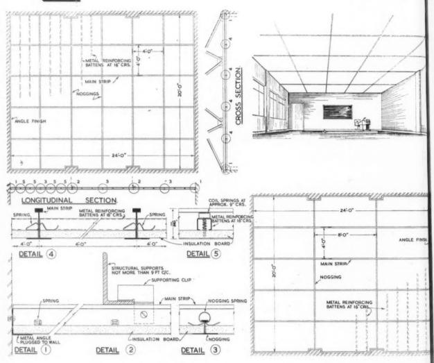
ARCHITECTS have often expressed the wish for a suspended ceiling construction embodying the advantages of our various Spring Clip systems but without the necessity of using cover strips at 2-ft. centres or less. The new TenTesT Construction illustrated above uses substantial extruded aluminium cover strips at 4-ft. centres and permits the use of panels from 4-ft. square up to 10-ft. long by 4-ft. wide. Sag in
