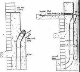
Details of rainwater disposal at edges and ends of barrel va
