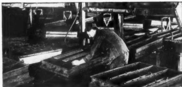
Part of the foundry in which the radiator moulds are formed. Photograph shows cores being placed in position.
