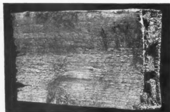
Fig. 6. Coniophora cerebella —cellar fungus—decay entirely internal.
