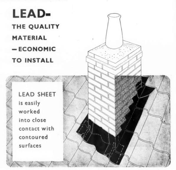
The intersection between chimney stack and roof is a weak point even in the best roof unless the flashings are sound and permanent. LEAD is the standard material for this purpose both because of the quality of the material itself and because of the ease with which it is fixed and worked into close contact jwith contoured surfaces. It is not corroded by town, rural or seaside atmospheres, nor by contact with other metals.
