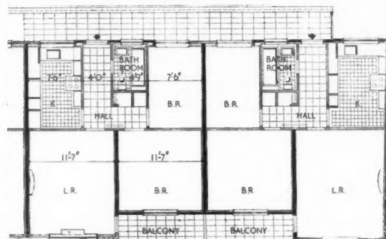
Plan of 3-room flat in 4 storey block [Scale: \frac{1}{4} " = 1' 0"]
