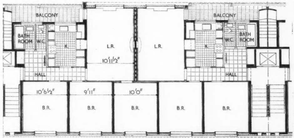
Plan of 3- and 4-room flats in 8-storey block [Scale: 1/2" = 1' 0"]
